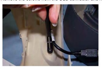
11. Attach the new USB cable to the connector and tighten the screws.
